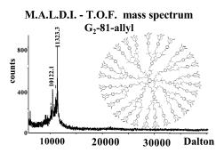
**Figure 3.** MALDI TOF mass spectrum of G<sub>2</sub>-81-allyl-dendrimer. The major peak is the molecular peak ( $M = 11\ 299$ ;  $[M + Na]^+$  at  $m/z\ 11\ 322$ ). The minor peak at 10 422 represents the same dendrimer in which one triallylphenol unit is missing, possibly because of the isomerization of a double bond during the catalyzed hydrosilylation reaction (see text).
