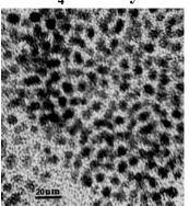
Figure 6. HRTEM picture of G<sub>4</sub>-729 coated with osmium oxide vapor and recorded on amorphous graphite support. Osmium oxide forms a fivemembered glycolate metallocycle by addition of the terminal double bonds of the branches onto oxo ligands<sup>37</sup> (the proportion of reacted terminal double bonds is unknown).
