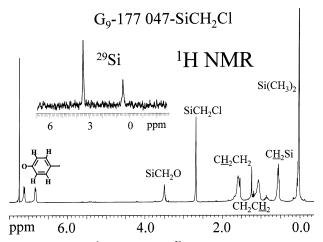
*Figure 2.* 400 MHz <sup>1</sup>H and 100 MHz <sup>29</sup>Si NMR spectra of G<sub>9</sub>-177 147-SiCH<sub>2</sub>Cl resulting from the catalyzed hydrosilylation of G<sub>9</sub>-177 147-allyl (see text). See the HRTEM of the iodo analogue in Figure 7.
