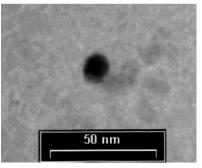
Figure 7. HRTEM picture of G<sub>9</sub>-177 047-SiCH<sub>2</sub>I recorded on amorphous graphite support showing the globular shape with a diameter of 13 nm (compare Table 1 and Figure 8) lower than that calculated (16.7 nm) for tethers with maximum extension. See the <sup>1</sup>H and <sup>29</sup>Si NMR spectra of the chloro analogue of this compound in Figure 2.
